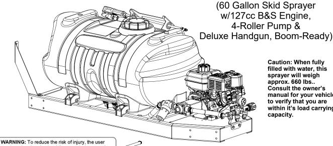
Caution: When fully filled with water, this sprayer will weigh approx. 660 lbs.. Consult the owner's manual for your vehicle to verify that you are within it's load carrying capacity.
